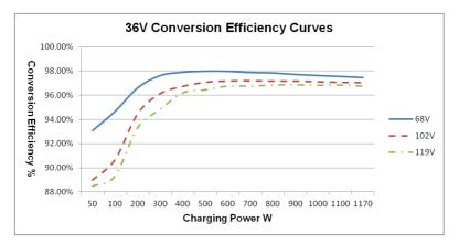
3. Solar Module MPP Voltage(68V, 102V, 119V) / Nominal System Voltage(36V)
