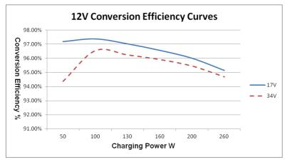
1. Solar Module MPP Voltage(17V, 34V) / Nominal System Voltage(12V)
